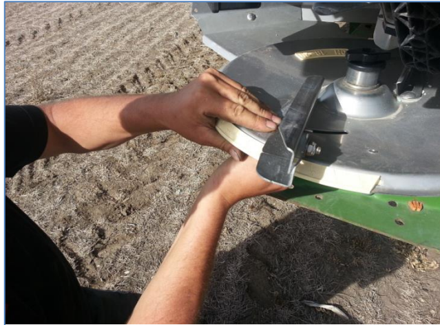
Image 5: Adjusting disc vane angle to alter spread pattern
