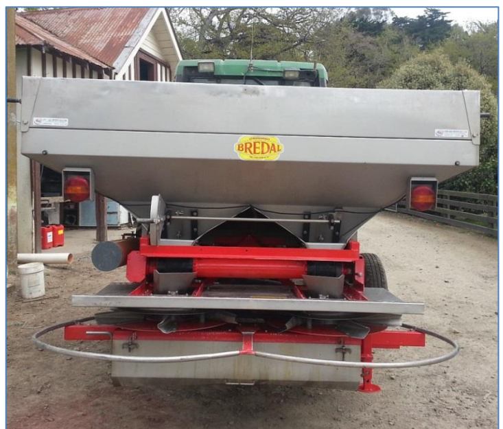
Image 2: Double disc spreader with contra-rotating discs for more even application
