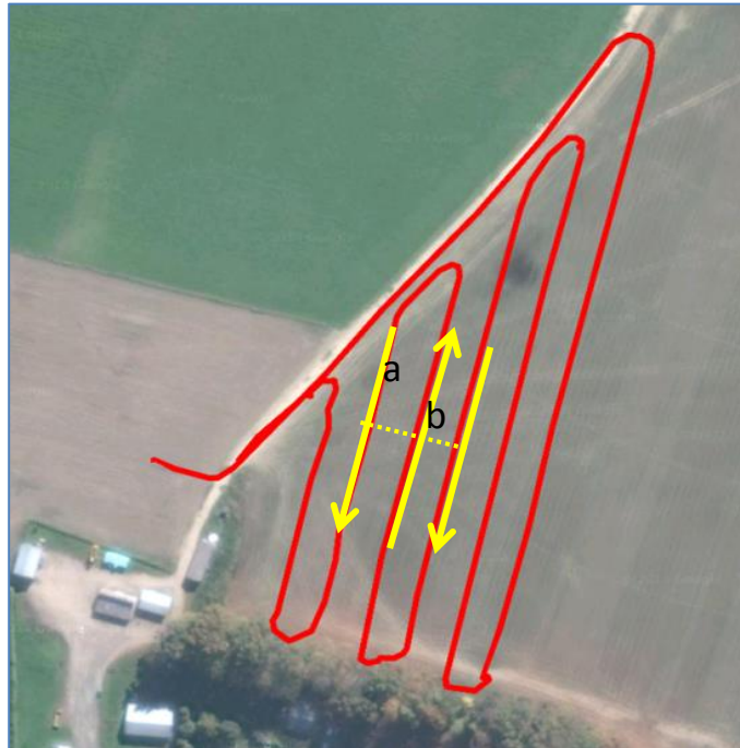
Figure 2 Tray layout and spreader runs for in-field overlap test
