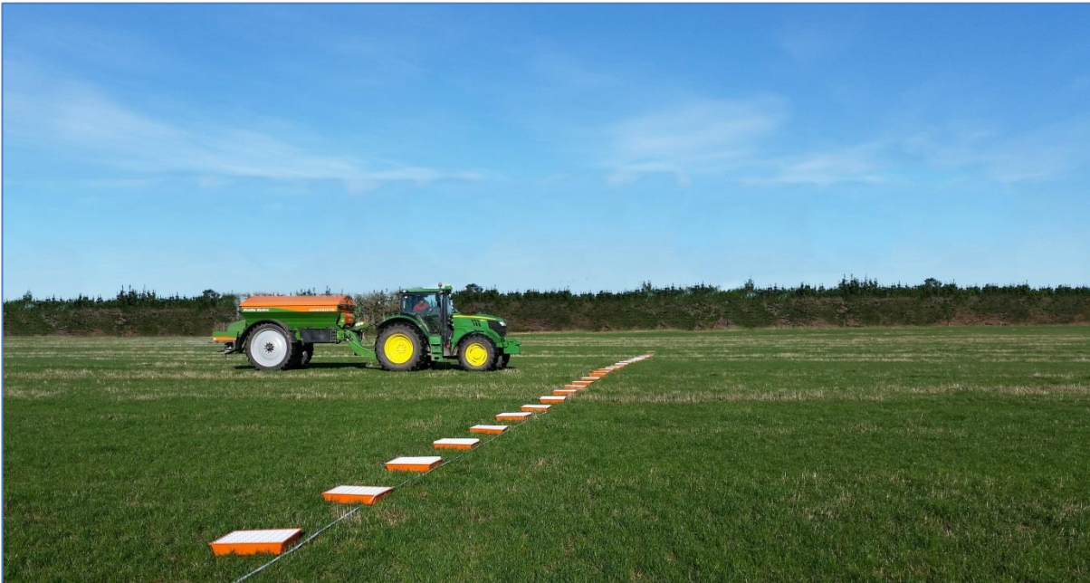
Image 10: A line of collection trays laid out across the fertiliser spreader travel path
