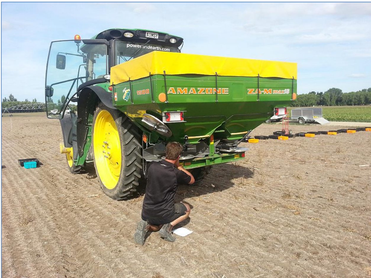
Image 4: Adjusting settings on double disk spreader
