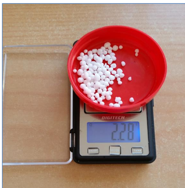
Image 11: Collected fertiliser sample being weighed on electronic scales
