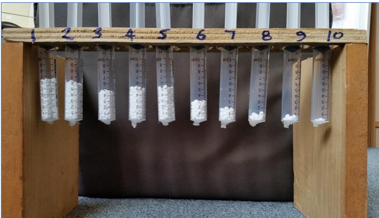
Image 13: A rack of graduated syringes acts as measuring cylinders and simply displays the application pattern
