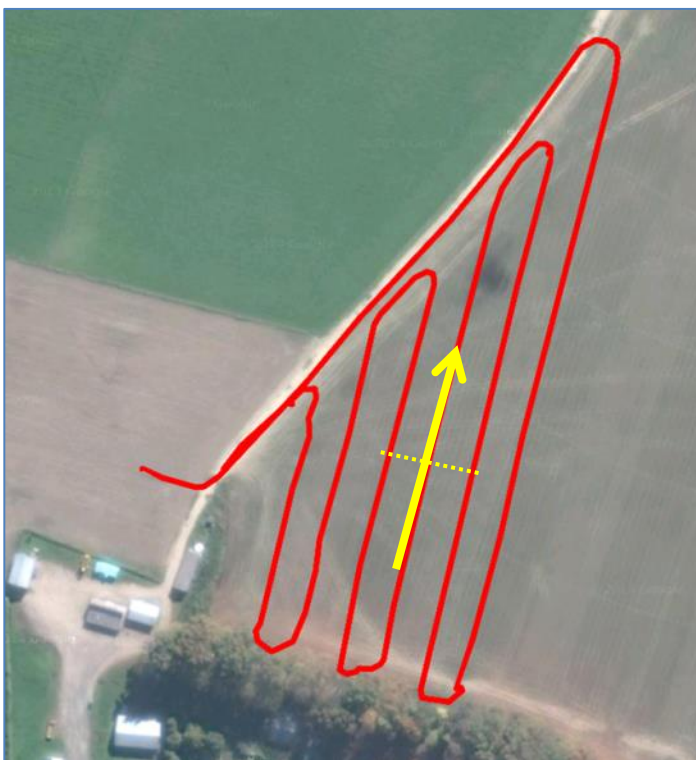
Figure 3 Tray layout and spreader run for a single pass test
